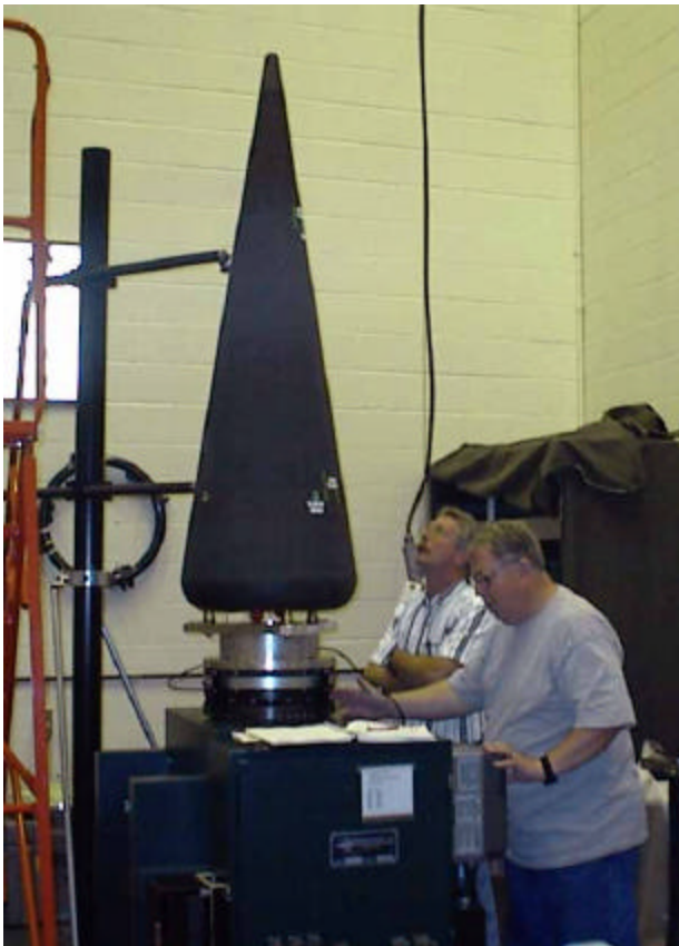
Figure 7 Using two dial indicators to adjust tilt
