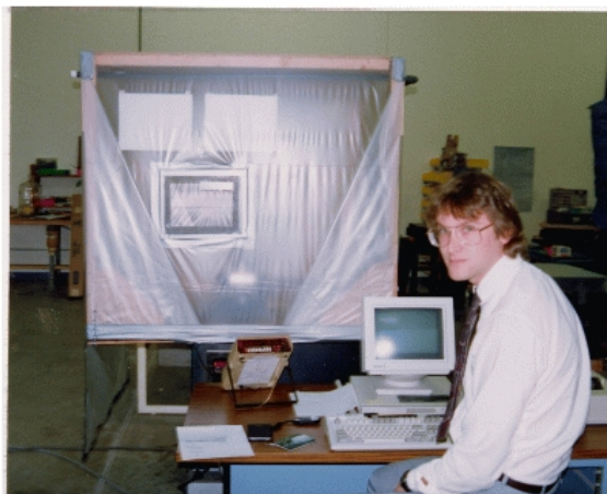
Figure 13A Operator and Helium Chamber
